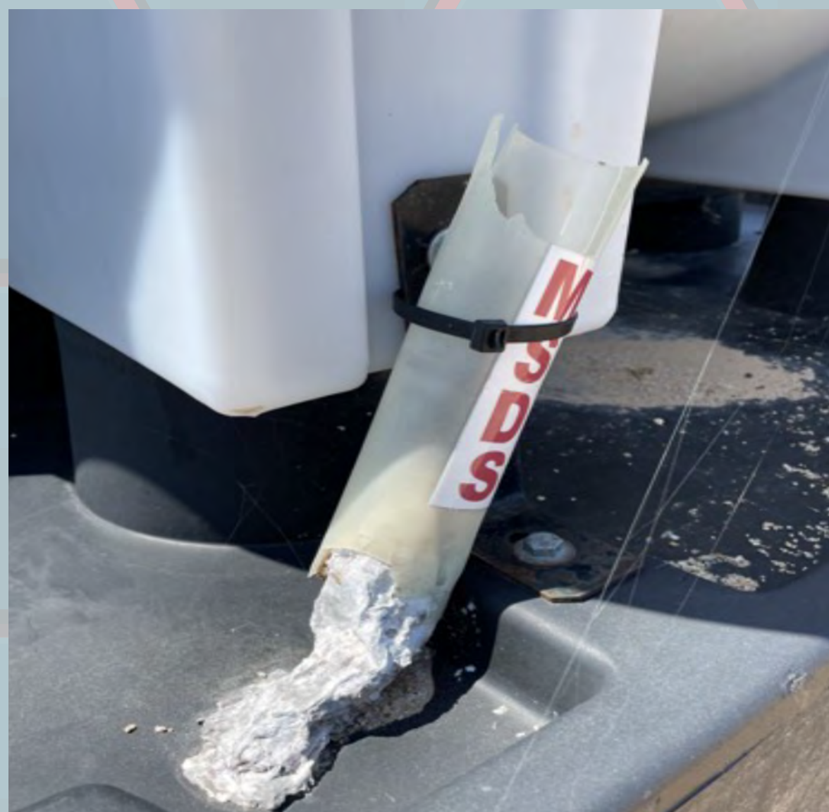
Picture 1: Shows disintegrated plastic tube with paper SDS severely damaged by weather.
